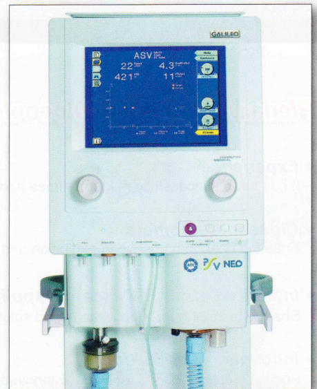
Figure 2. The first device ever to incorporate ASV was the Galileo ventilator launched in 1998.
