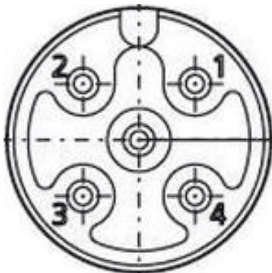
Fig. 7 M12 A-coded Male Pinout (front view)
