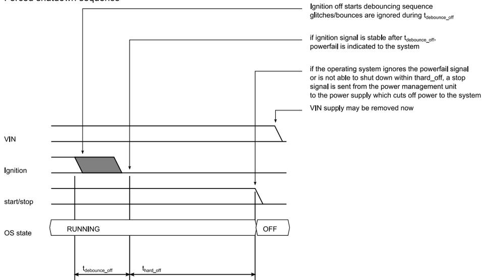
Fig. 25 Shutdown timing diagram
