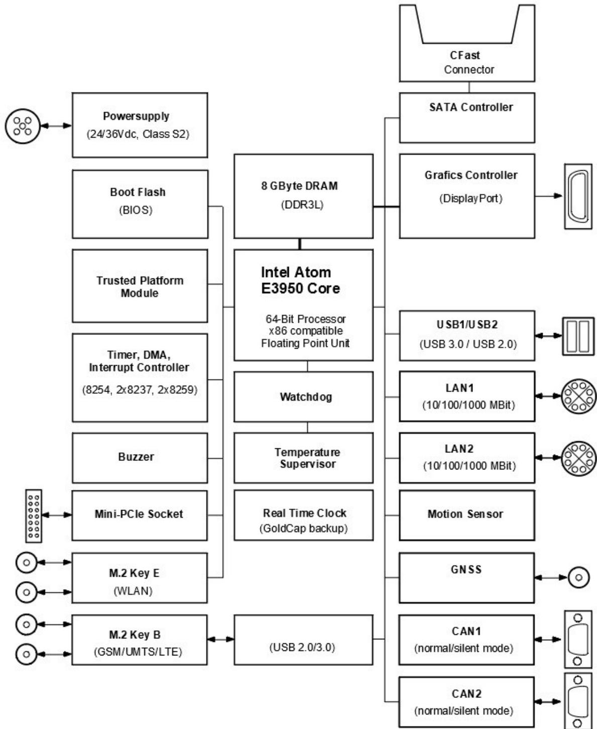
Fig. 1 Block Diagram RSL81 (IPC/RSL81120-R152E shown)
