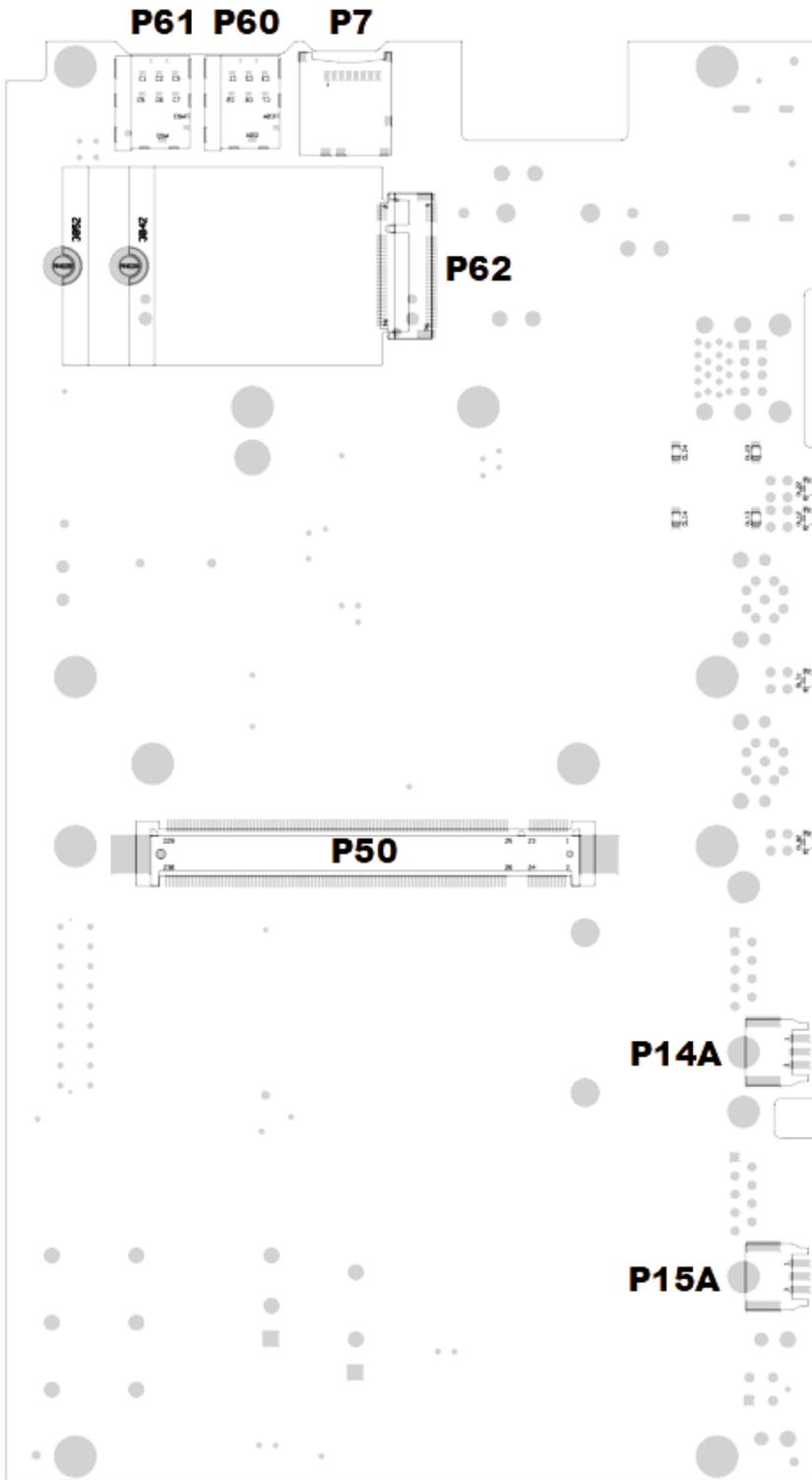
Fig. 11 Board Layout RSL81 Baseboard Bottom Side
