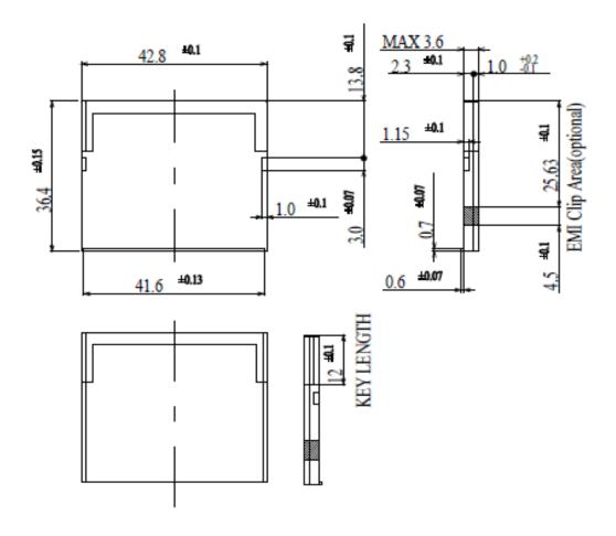
Figure 2-1. Type I CFast Card Dimensions
