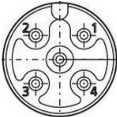
Fig. 7 M12 A-coded Male Pinout (front view)
