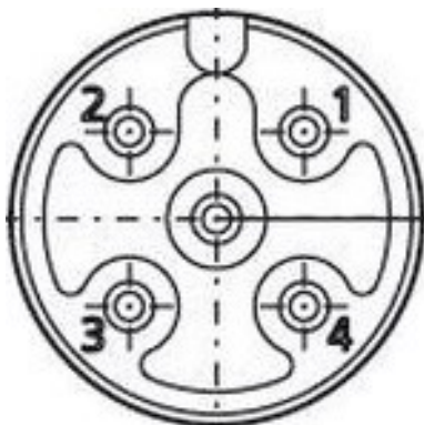
Fig. 7 M12 A-coded Male Pinout (front view)
